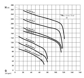
H = Total Head; Q = Discharge Volume. Curves to Hydraulic Institute N.B. please use the ABSEL program to validate pump selection.
